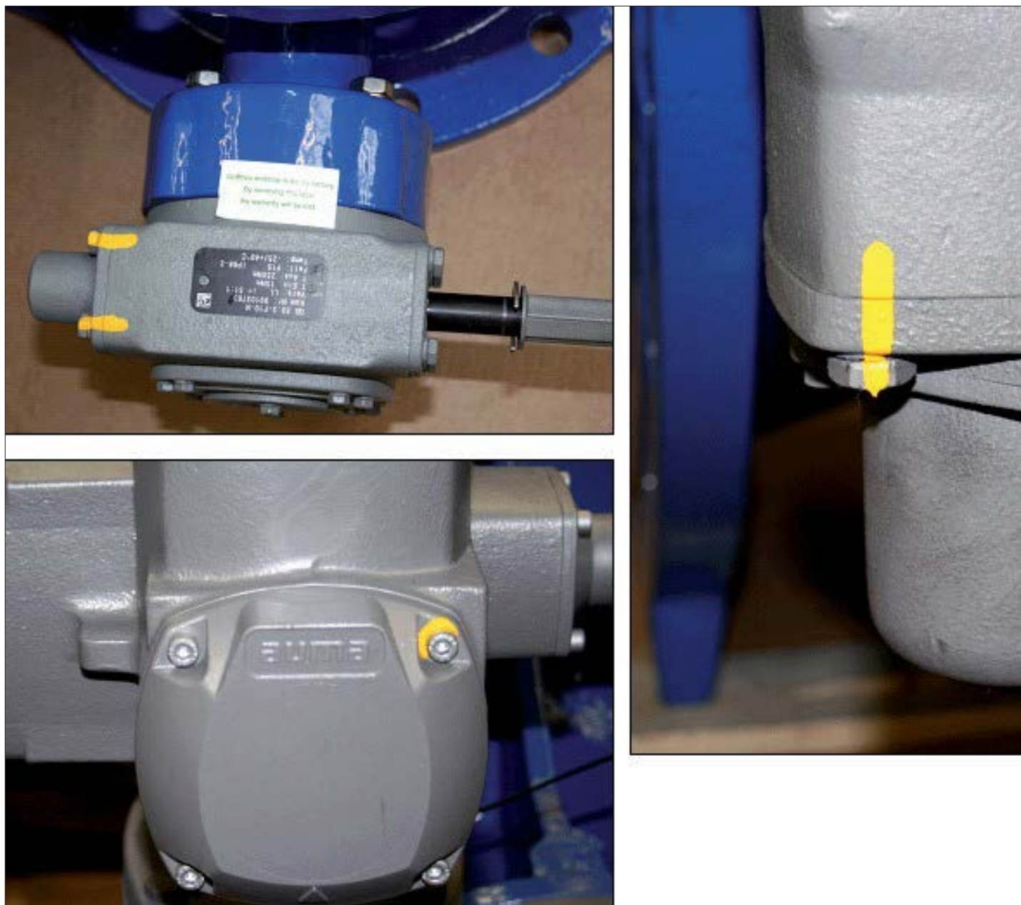
Figure 12: Markings on the gear unit
